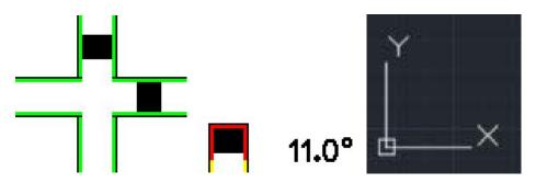
X & Y axis of machine where is X is left to right of machine and Y is front to back. The positive angle will be shown which will be shown on the position where the machine is highest. The position of the cursor moves towards the high angle.
